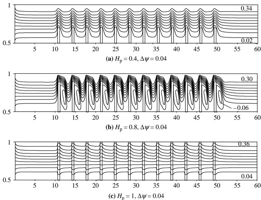
**Figure 5.** Effects of the porous fins height on streamlines for  $L_f = 3$  and  $Da = 10^{-5}$
