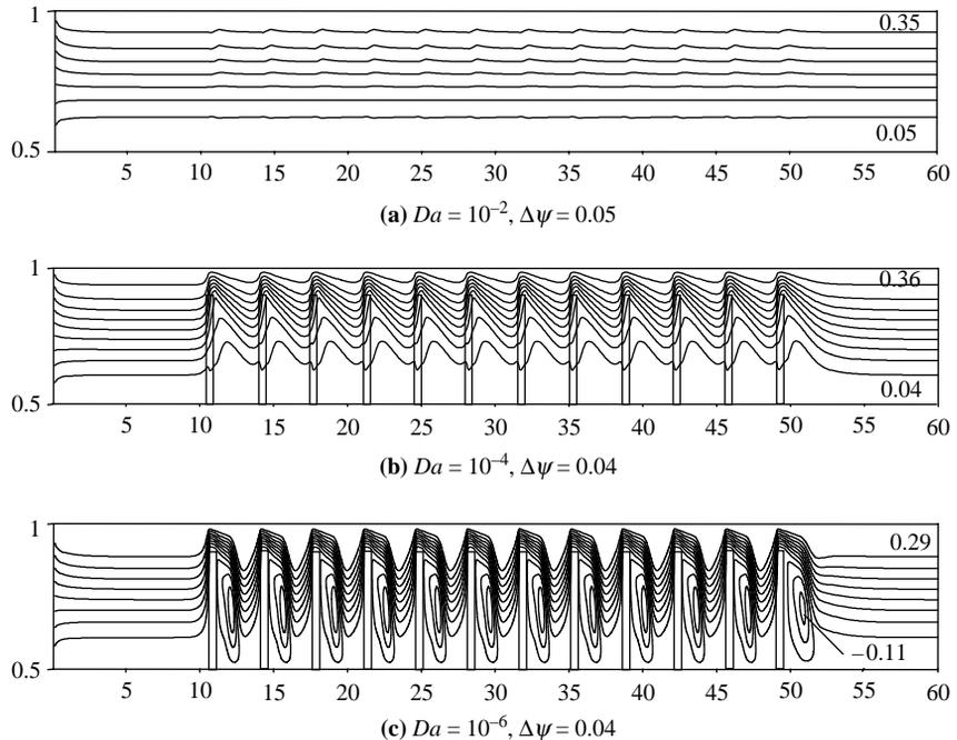
**Figure 4.** Effects of the Darcy number on streamlines for  $L_f = 3$  and  $H_p = 0.8$
