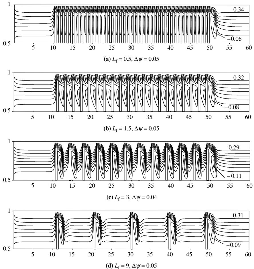
**Figure 6.** Effects of the porous fins spacing on streamlines for  $H_p = 0.8$  and  $Da = 10^{-6}$
