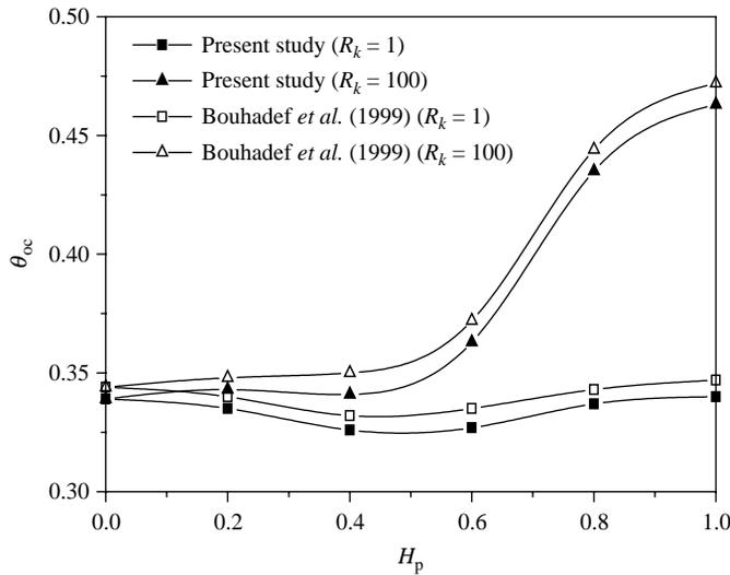
**Figure 2.** Outlet temperature of the cold fluid as function of  $H_p$  and  $R_k$ :  $Re = 100$ ,  $Pr = 4$ ,  $L = 50$  and  $Da = 10^{-2}$
