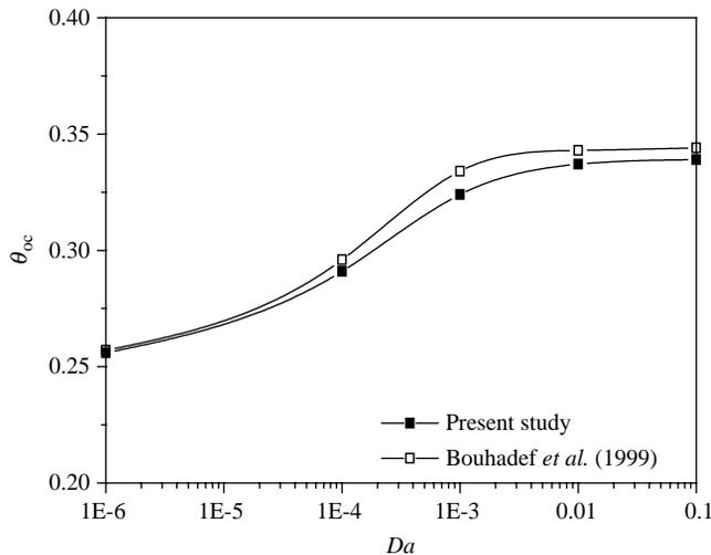
**Figure 3.** Outlet temperature of the cold fluid as function of  $Da$ :  $Re = 100$ ,  $Pr = 4$ ,  $L = 50$  and  $H_p = 0.8$
