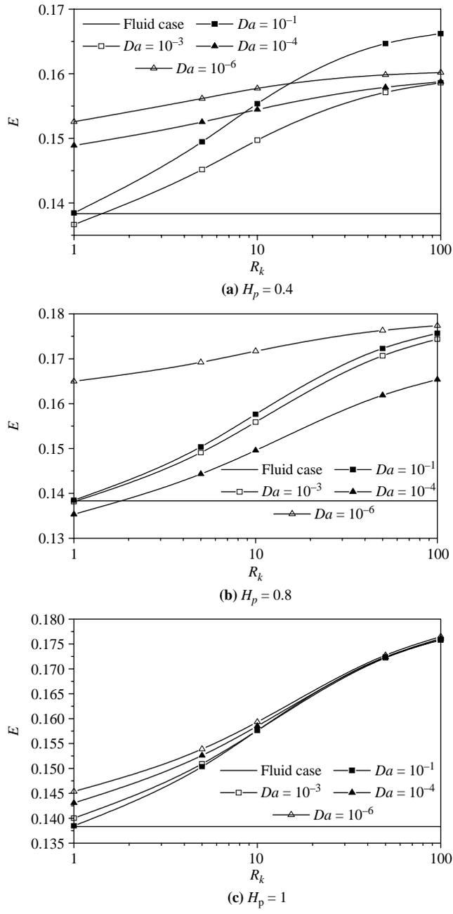
**Figure 10.** Heat exchanger effectiveness versus thermal conductivity ratio for  $L_t = 3$
